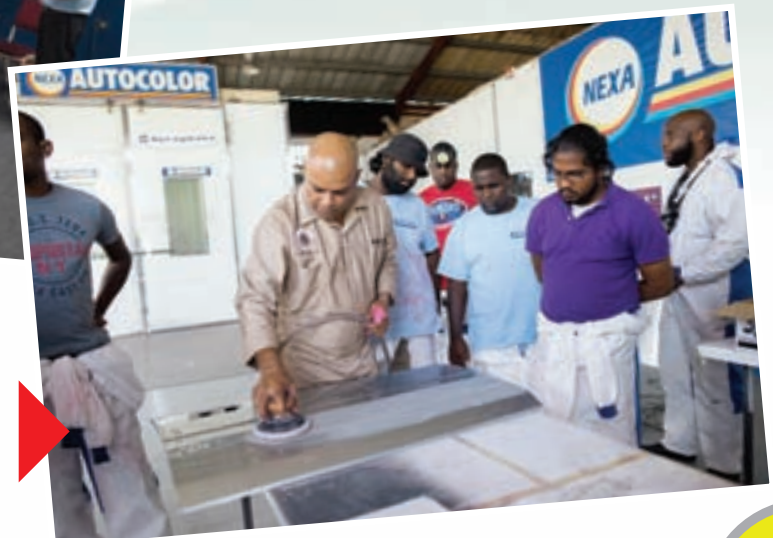
Mr. Talaat Mohammed demonstrates sanding the door of a vehicle before it is sprayed with paint, as part of surface preparation
